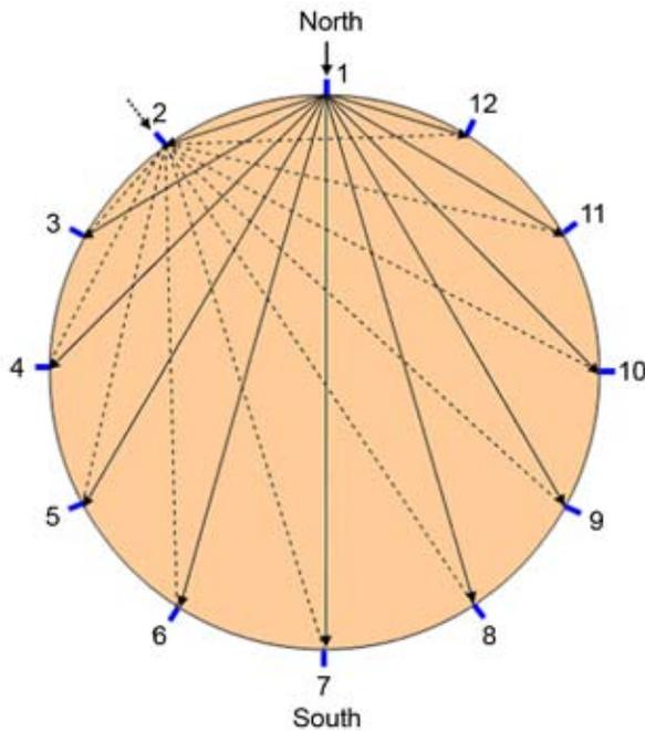
**Figure 1. Sensor arrangement on a tree trunk for acoustic tomography measurement on trees.**
