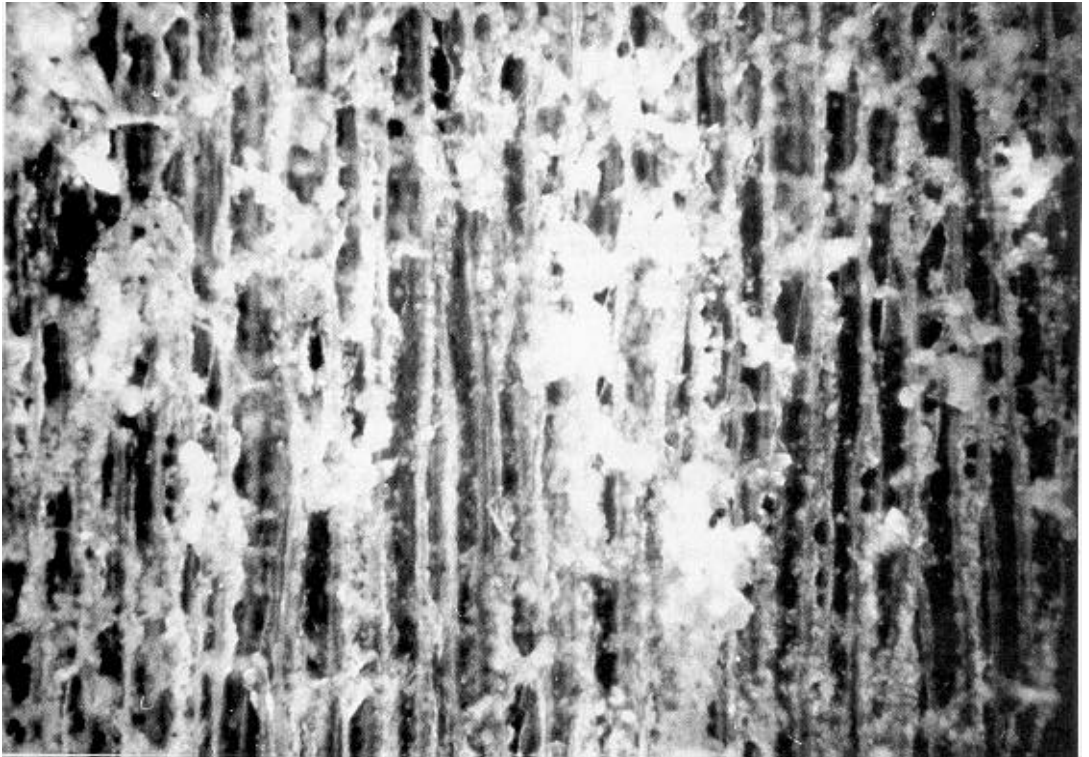
Figure 1—Surface view of a broken joint with no visible glue film; only the filler is visible. (M90 0037-19)
