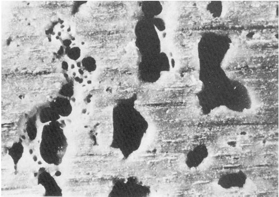
Figure 7—Surface-view micrograph of a broken joint showing a thick glueline with large voids. This glueline was formed without adequate pressure. (M90 0037-7)
