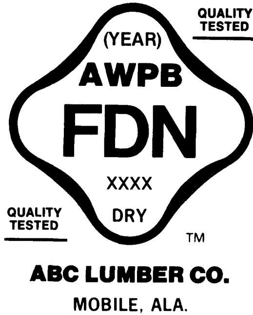
Figure 1.--An example of the AWPB, FDN stamp that is required on each piece of plywood and treated lumber in wood foundations.
