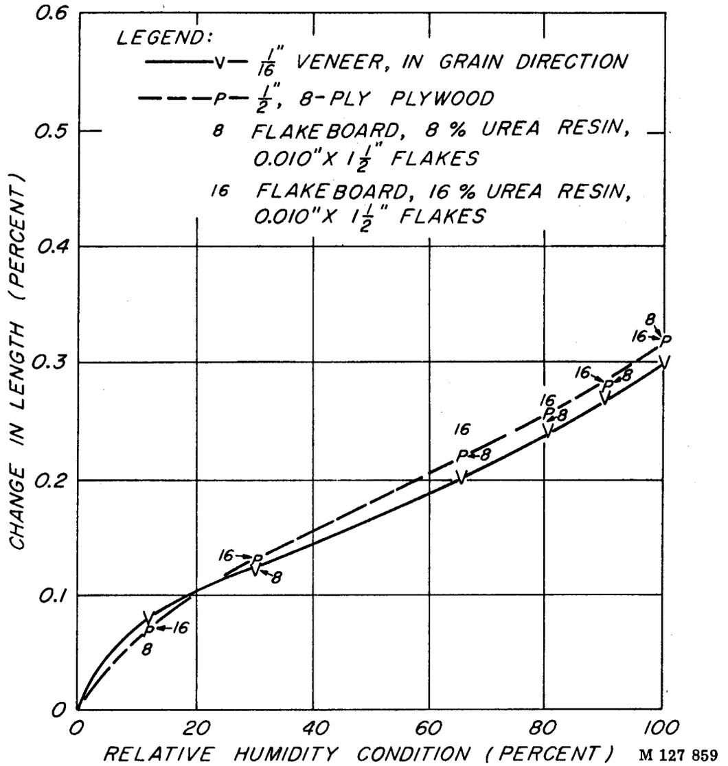
Figure 5.--Aspen: Linear movement of veneer, plywood, and flakeboards as related to change in moisture content from oven-dry condition.
