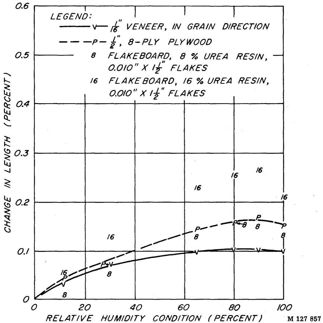
Figure 7.--Douglas-fir: Linear movement of veneer, plywood, and flakeboards as related to change in moisture content from oven-dry condition.
