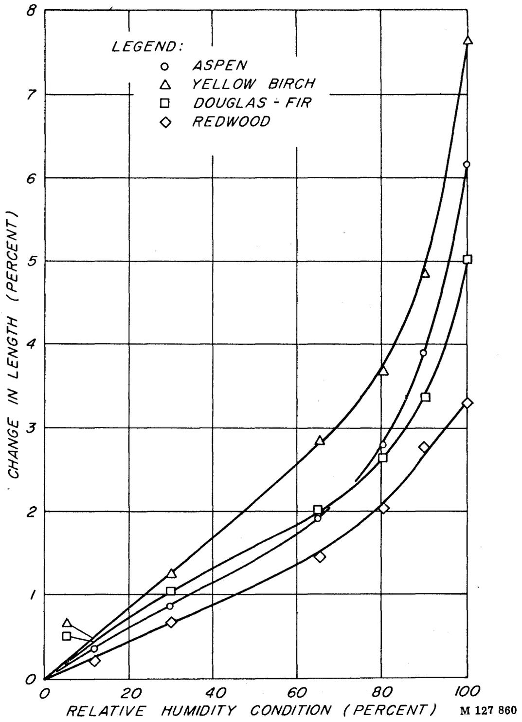
Figure 4.--Transverse-to-grain movement of veneer as related to change in moisture content from oven-dry condition.
