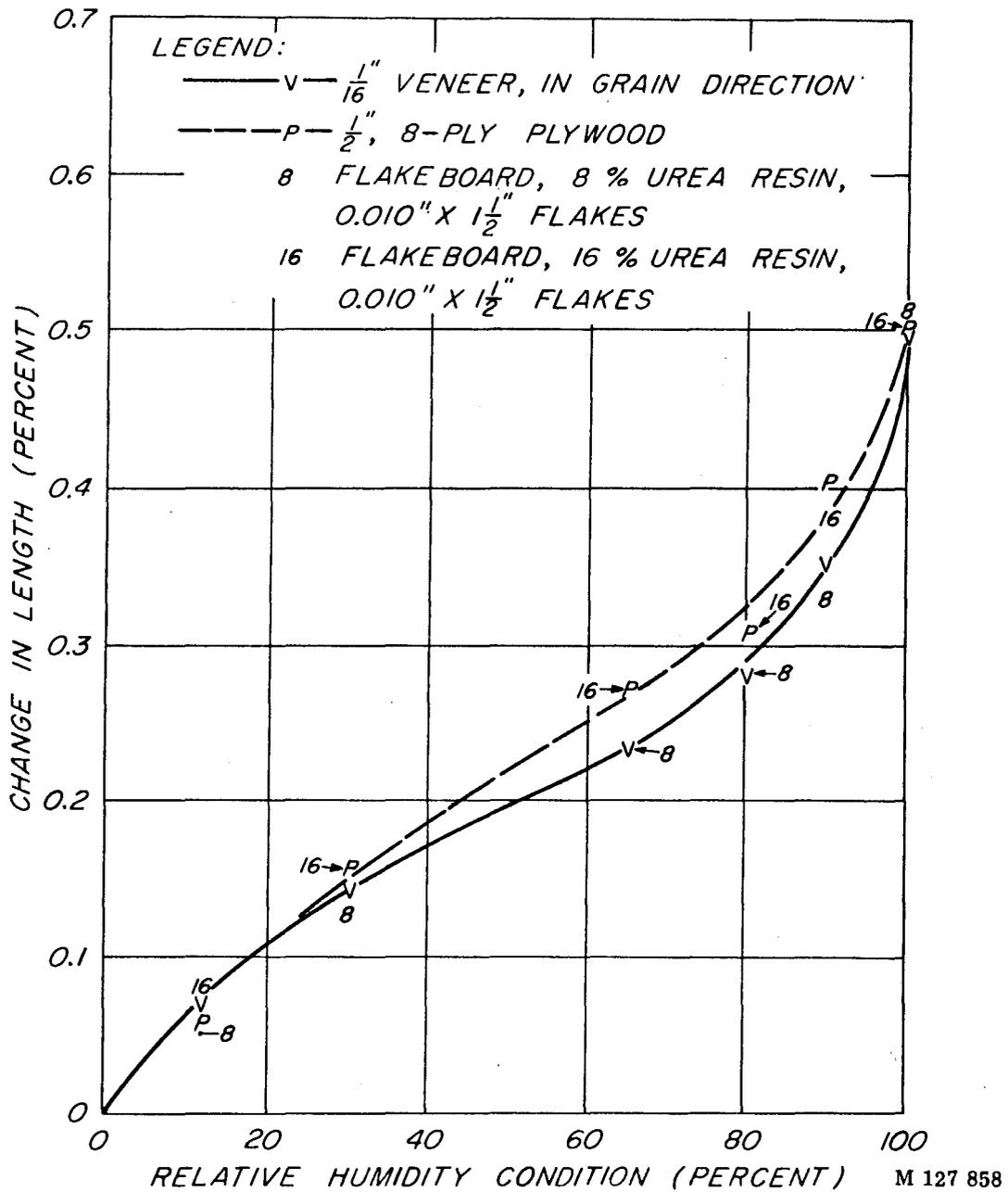
Figure 6.--Yellow birch: Linear movement of veneer, plywood, and flakeboards as related to change in moisture content from oven-dry condition.
