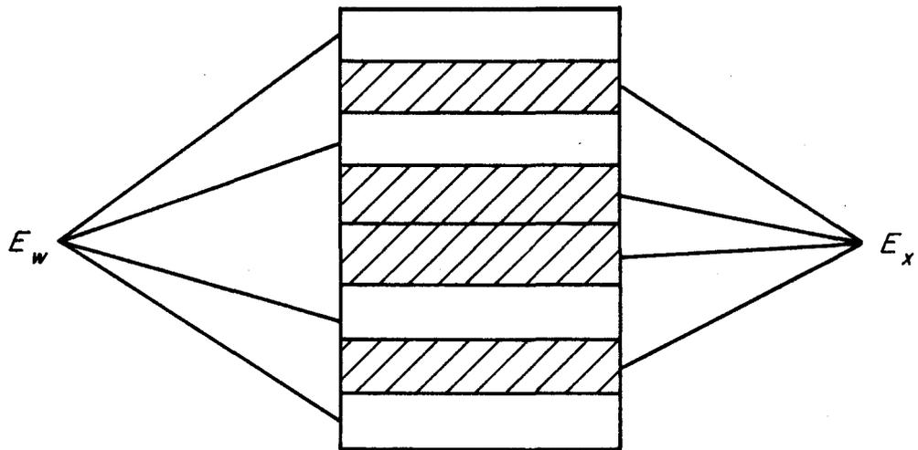
Figure 13.--Section of 8-ply 50-50 construction plywood.
