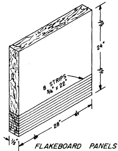
Figure 2.--Specimen cutting diagrams. M127 862
