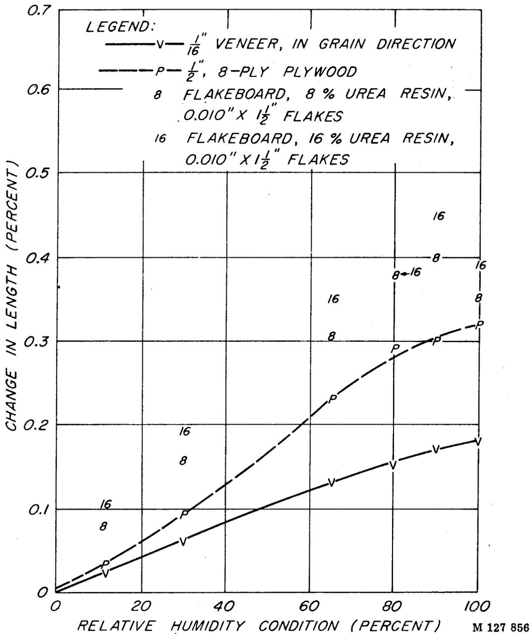
Figure 8.--Redwood: Linear movement of veneer, plywood, and flakeboards as related to change in moisture content from oven-dry condition.
