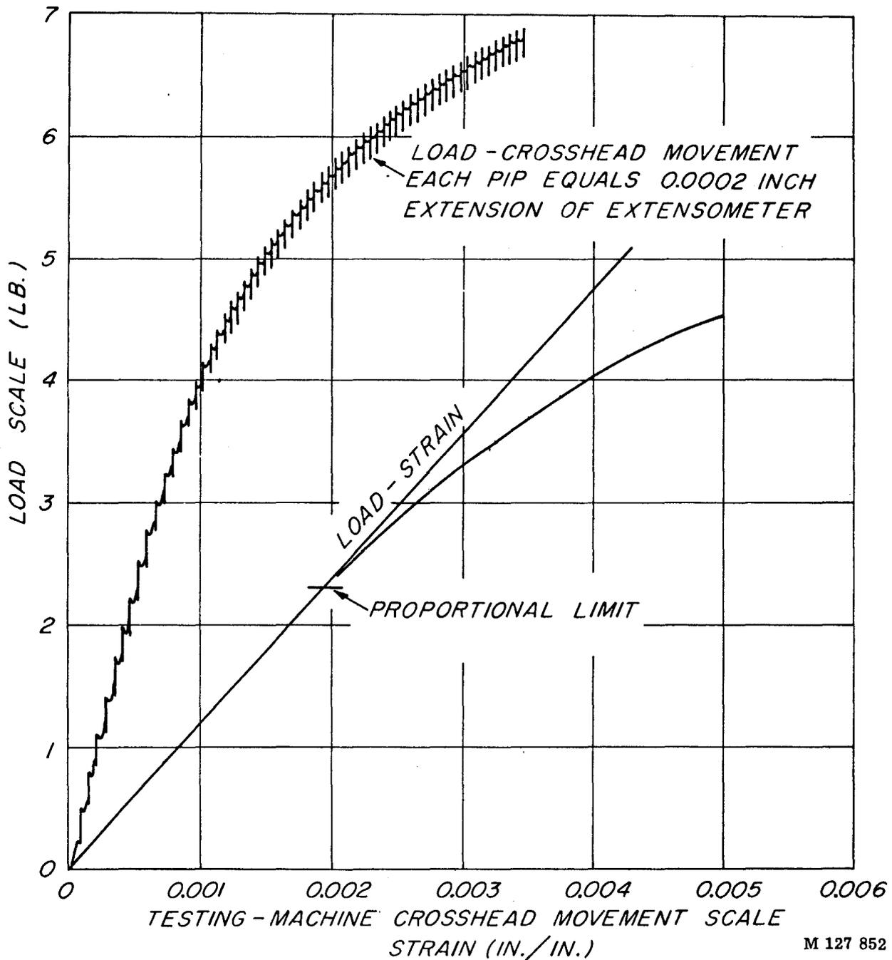
Figure 12.--Example of autographing record obtained from testing machine. Vertical marks or pips were inserted by operator reading extensometer gage.
