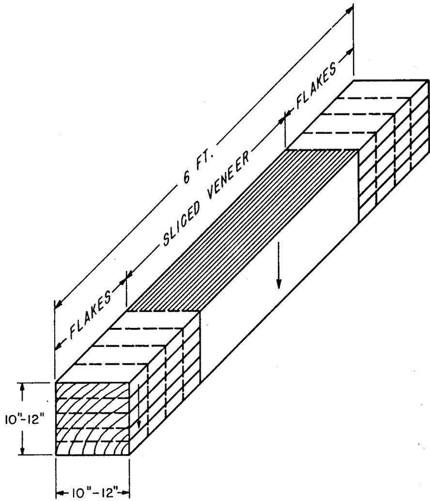
Figure 1.--Cutting diagram of flitch.
