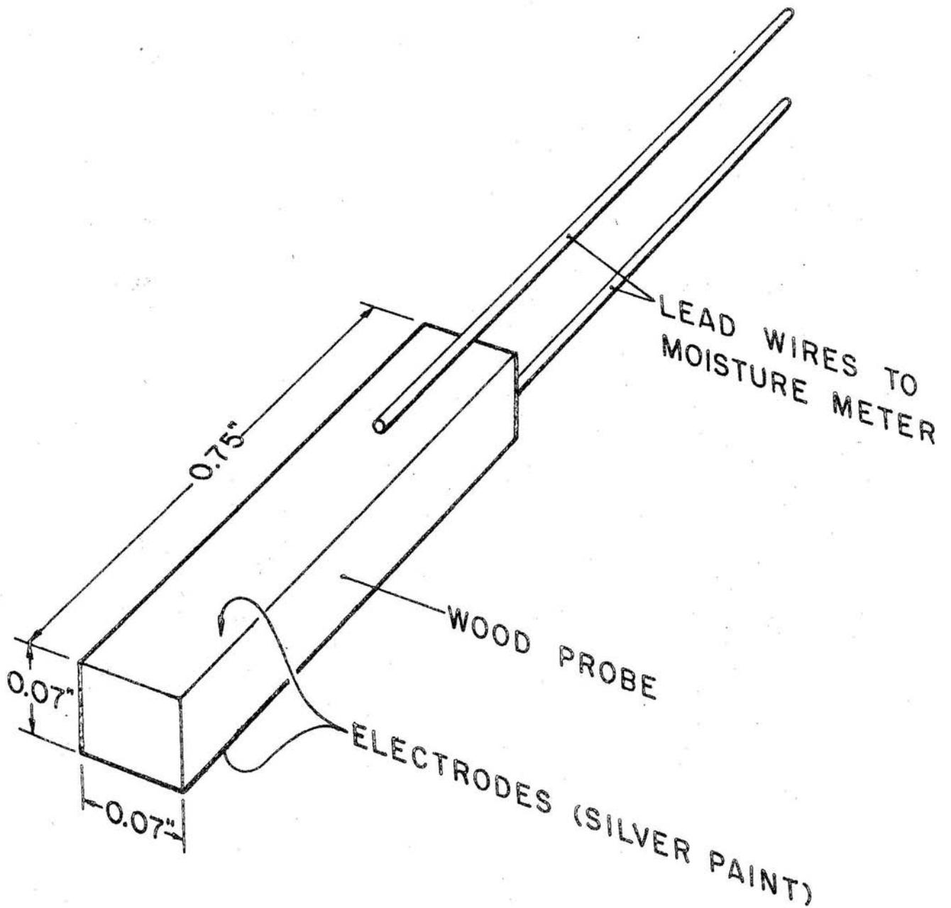
To design a direct-reading moisture probe from wood material, knowledge of the relationship between the geometry and the electrical resistance of the probe is required. In general, the electrical resistance of the probe follow the equation:<sup>2</sup>
