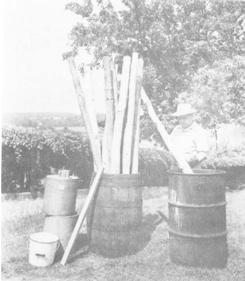
Figure 1. -- All of the equipment needed to treat fence posts by double diffusion is shown here.
