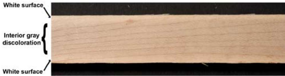
Figure 4. Edge view of board with white surfaces but with interior gray discoloration.
