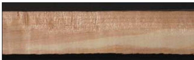
**Figure 3. Edge view of board showing blotchy red discoloration in soft maple board treated with sulfur dioxide.**
