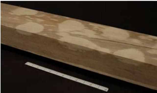
Figure 6. Hammer impact in ochoó board marked by *unstained* (white) wood.
