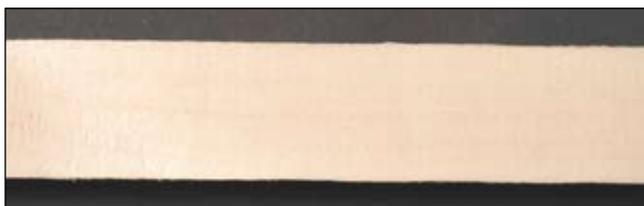
**Figure 1. Edge view of pure white soft maple board treated with sulfur dioxide.**
