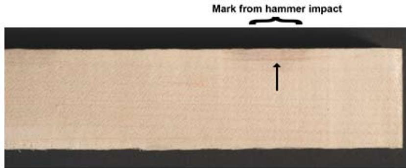
Figure 5. Edge view of soft maple board showing hammer impact marked by discolored wood.
