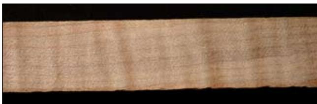
**Figure 2. Edge view of board showing severe gray discoloration in untreated soft maple board.**
