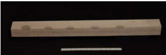
Figure 7. Hammer impacts in soft maple board marked by *stained* wood.
