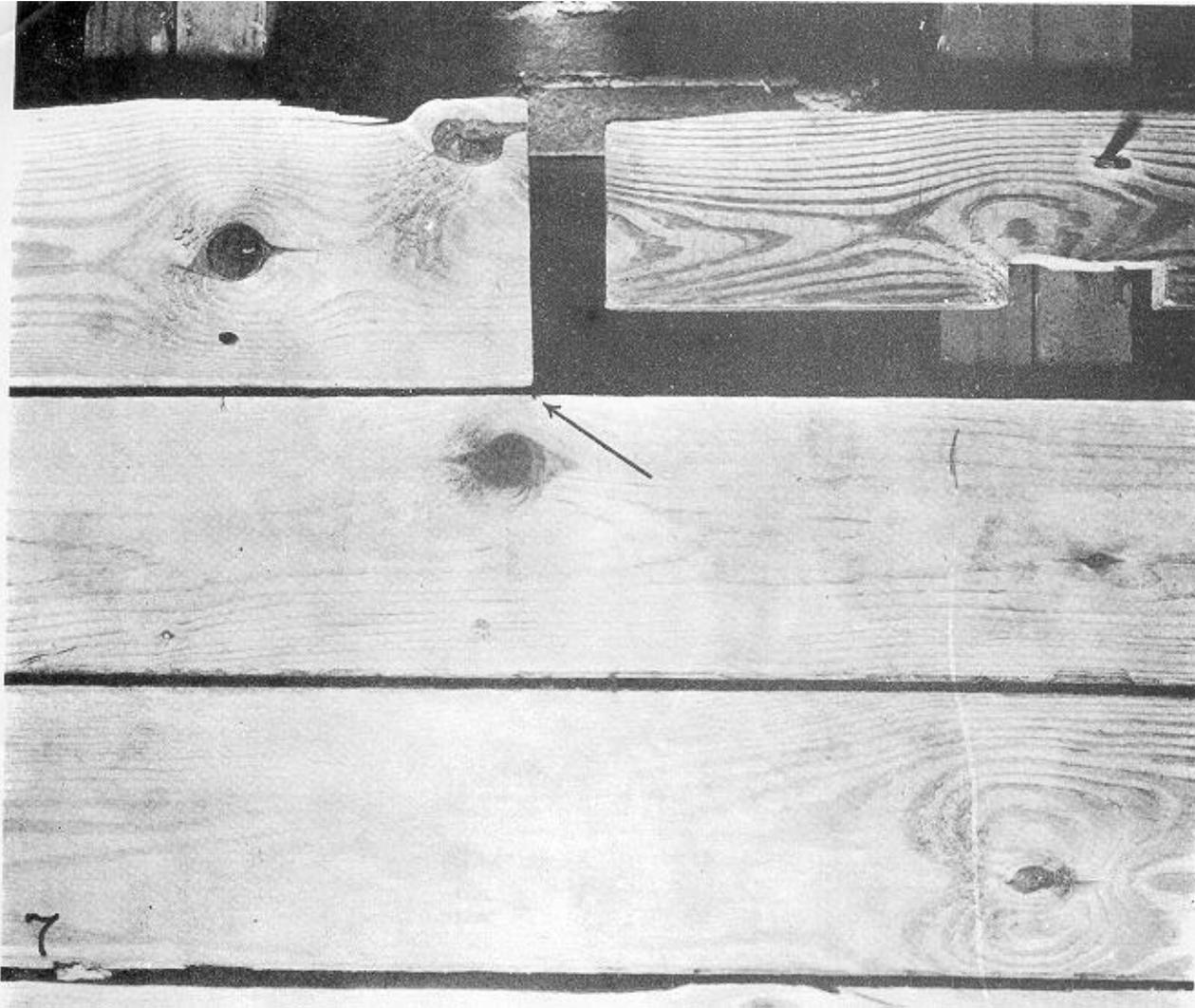
Figure 7 --End of discontinuous attic floor board (left) as found in Hamptmann's attic and of ladder rail No. 16 (right) replaced in its original position. That the rail was made from a piece of a board removed from the attic floor is indicated by the following facts:
