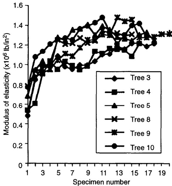
Figure 4—Red alder modulus of elasticity at breast height. The specimen numbers begin at the pith and increase toward the bark from left to right.
