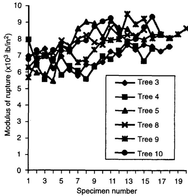
Figure 5—Red alder modulus of rupture at breast height. The specimen numbers begin at the pith and increase toward the bark from left to right.
