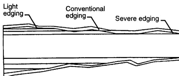
Figure 1—Edger line locations for light, conventional, and severe edging.
