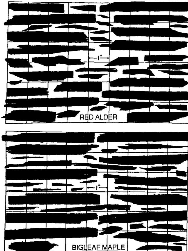
Figure 1—Typical flake dimensions.
