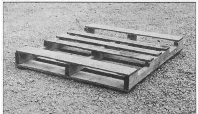
**Figure 1—Top and bottom decks of a test pallet.**
