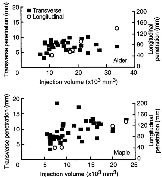
Figure 1—Injection water volume (after 10 seconds) versus transverse and longitudinal preservative penetration for alder (top) and maple (bottom).
