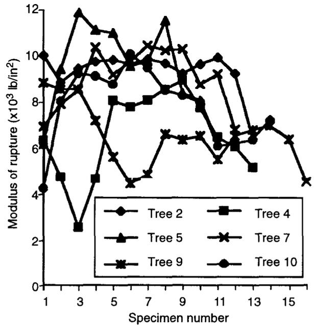
Figure 10—Oregon white oak modulus of rupture at breast height. The specimen numbers begin at the pith and increase toward the bark from left to right.
