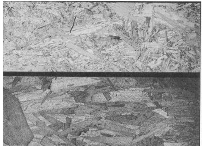
Figure 2—Oriented strand lumber panels using bigleaf maple (top) and red alder (bottom).
