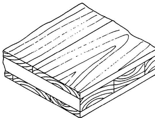
**Figure 1—Typical blockboard produced in this study.**
