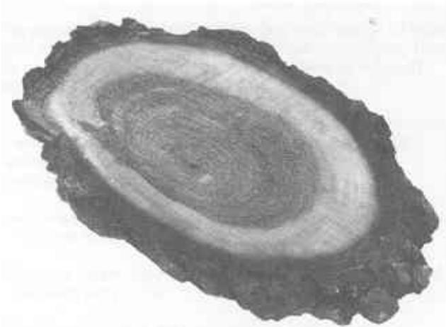
Figure 1—Cross section of walnut treated with polyethylene glycol (PEG). PEG-treated wood resists cracking and retains its bark. (M 87 0065)
