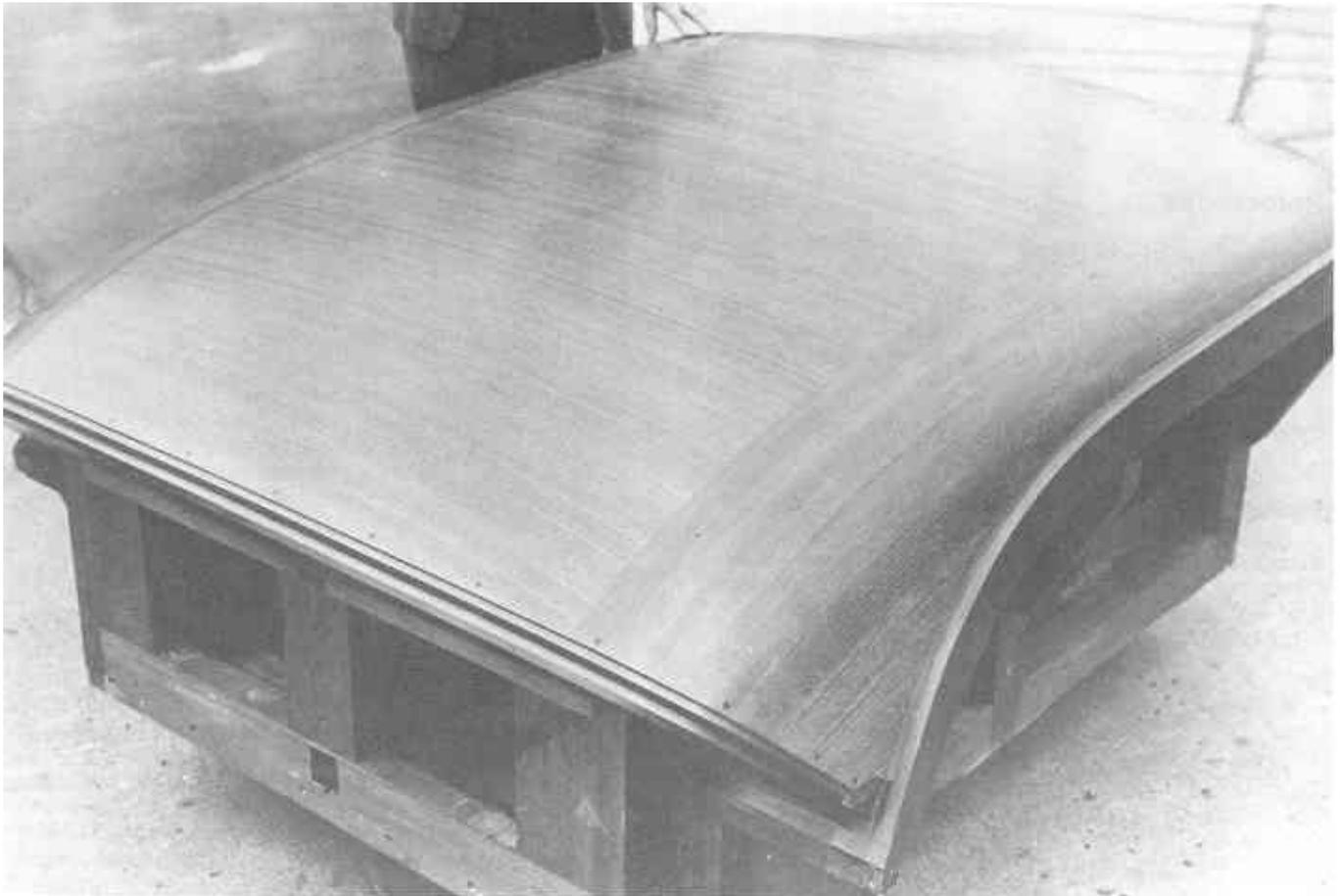
Figure 2—Roof master die model made from mahogany Impreg. impreg is workable and has dimensional Stability. (M 96073 F)
