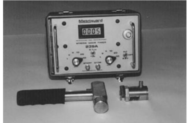
Figure 9—Metriguard Model 239A Stress Wave Timer.
