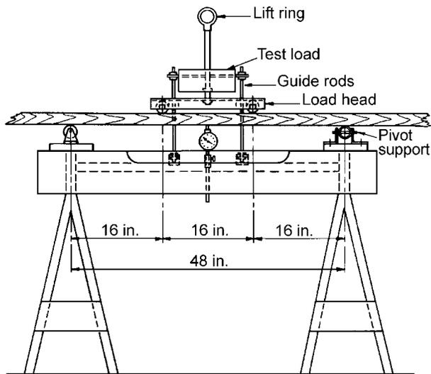
**Figure 8—Static tester.** This simple mechanical device applies a dead load to a piece of lumber placed flat on a 4-ft span.
