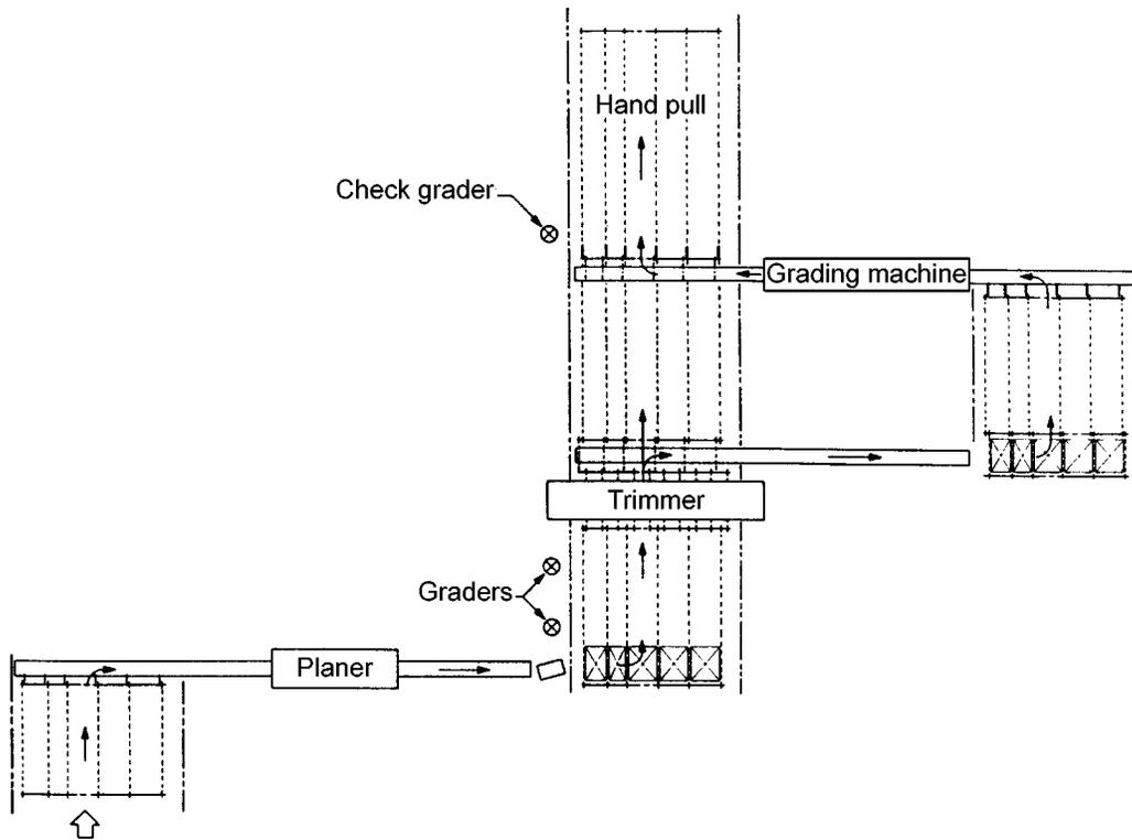
**Figure 18—Basic planing mill arrangement for machine grading. Visual graders designate pieces to be routed through grading machine. Check grader follows machine grading and trimming operation to assure correct grade output. Only a portion of lumber normally passes through grading machine.**
