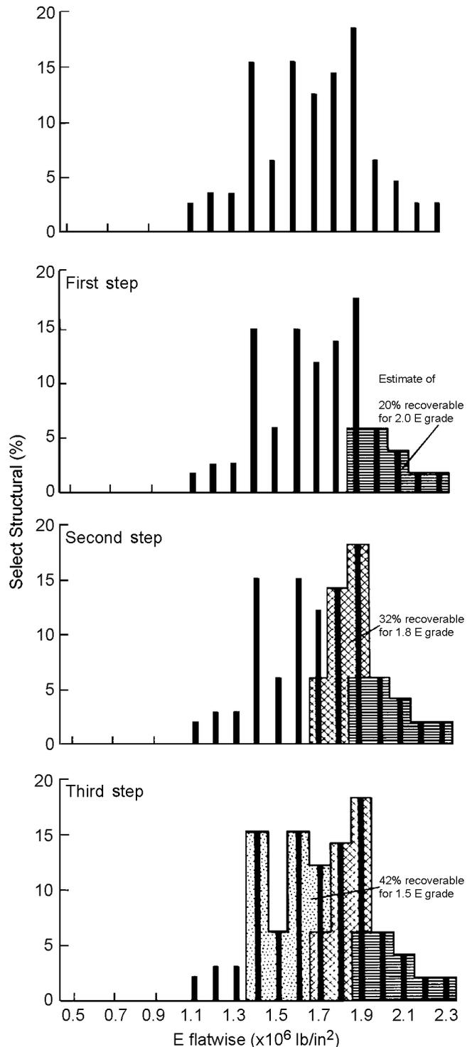
**Figure 15—Procedure for estimating fraction of Select Structural 2 by 4’s recoverable by E measurement. Data from Figure 10, combined results.**
