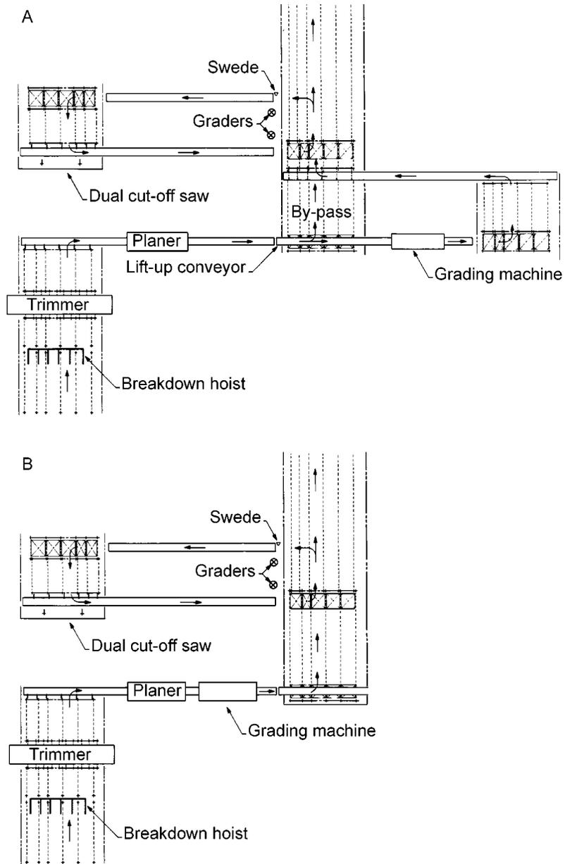
**Figure 25—Planing mill arrangement in which all lumber is trimmed before planing and passed through the grading machine as standard procedure. The by-pass (A) permits mill operation with visual grading if the grading machine is out of operation or is not needed. Part B illustrates close coupling to the planer.**
