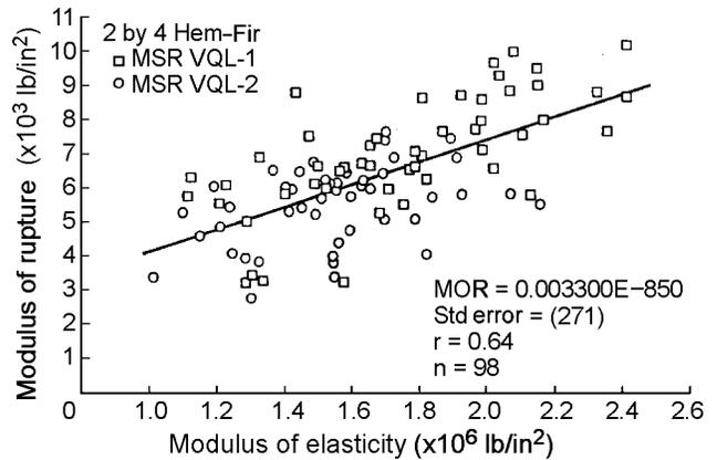
**Figure 13—Relationship between modulus of rupture (MOR) and flatwise modulus of elasticity (E), as measured by static tester.**
