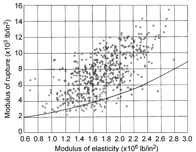
Figure 2—Typical relationship between strength predictor, MOE, and strength. The tolerance limit assures that about 95% of the data will fall above the line.
