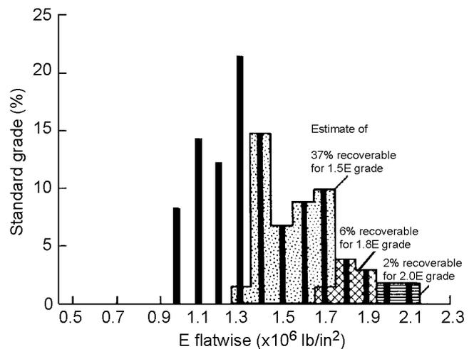
**Figure 17—Estimate of fraction of Standard grade 2 by 4's recoverable by E measurement. From Fig. 12, combined data, using procedures shown in Fig. 15.**
