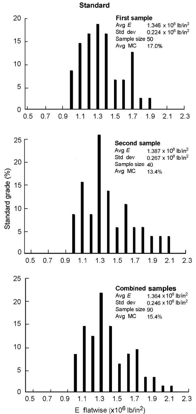
**Figure 12—Flatwise E of 2 by 4 Standard grade lumber, as measured by static tester. Results for two individual samples and combined samples.**
