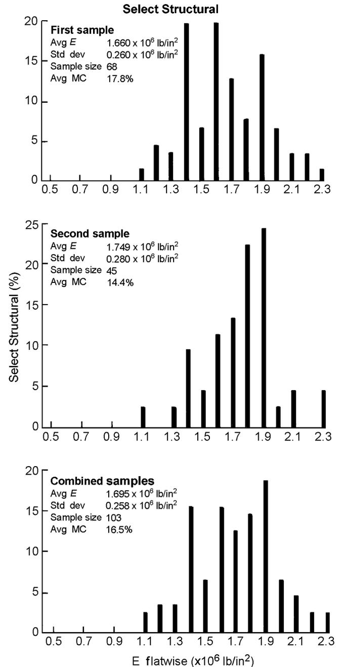
**Figure 10—Flatwise E of 2 by 4 Select Structural lumber, as measured by static tester. Results for two individual samples and combined samples.**
