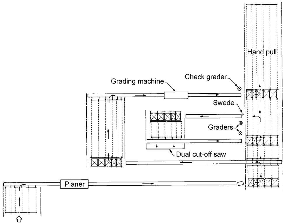
Figure 24—Planing-grading operation in which all trimming is handled by dual a cut-off saw.
