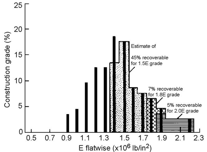
**Figure 16—Estimate of fraction of Construction grade 2 by 4's recoverable by E measurement. From Fig. 11, combined data, using procedures shown in Fig. 15.**
