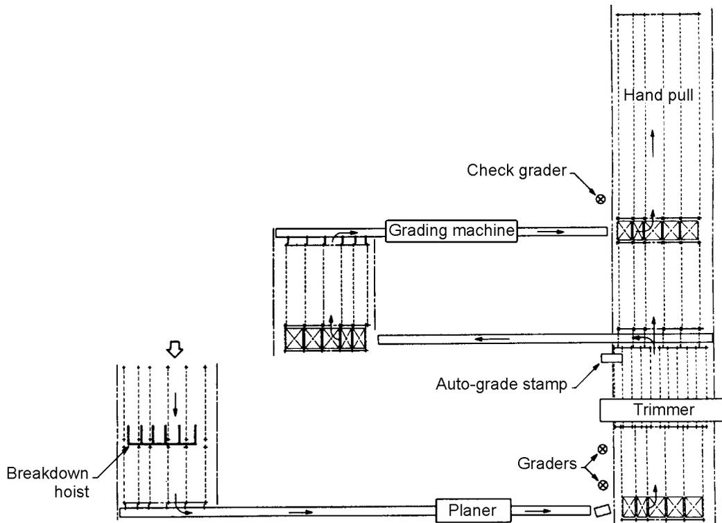
**Figure 19—Mill grading arrangement modified from that of Figure 28 to incorporate automatic grading-trimming station that also controls lumber to be routed to grading machine.**
