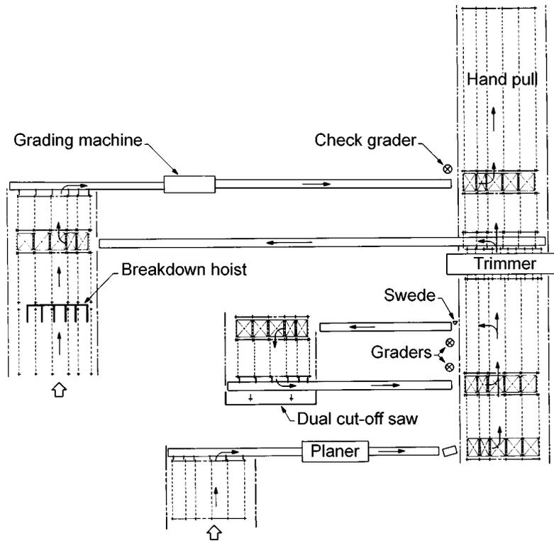
**Figure 20—Planing mill arrangement in conjunction with grading machine. Graders can use cut-off saw to upgrade lumber prior to final visual or machine grading. Arrangement includes separate breakdown hoist that permits machine grading independent of standard planing–grading–trimming operation.**
