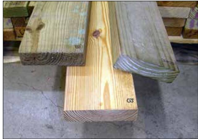
**Figure 3. (From left to right) Wood treated with MCQ, DDAC, and ACQ. Cupric ions from the wood preservative causes the dark coloration of the wood. Excess copper has deposited on the MCQ (green splotches) and the ACQ (along the end grain).**
