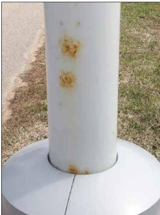
**Figure 11.** Corrosion underneath a coating failure. This lamp post was in service for less than 5 years before corrosion was visible at defects in the coating.
