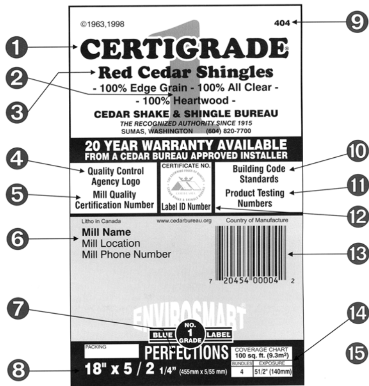
Figure 1. Information on a Certi-Label™: 1) “Certi” brand name; 2) Product grade; 3) Product type; 4) Independent third party quality control agency; 5) Compliance with total quality processes; 6) Manufacturer; 7) Industry product description; 8) Product dimensions; 9) Cedar Shake and Shingle Bureau label number; 10) Building code compliance numbers; 11) Product performance tests passed; 12) Label identification number; 13) UPC code; 14) Coverage showing the number of bundles/100 square-feet and recommended exposure; 15) Application instruction on reverse side. Used with permission from Cedar Shake and Shingle Bureau Exterior and Interior Wall Manual .
