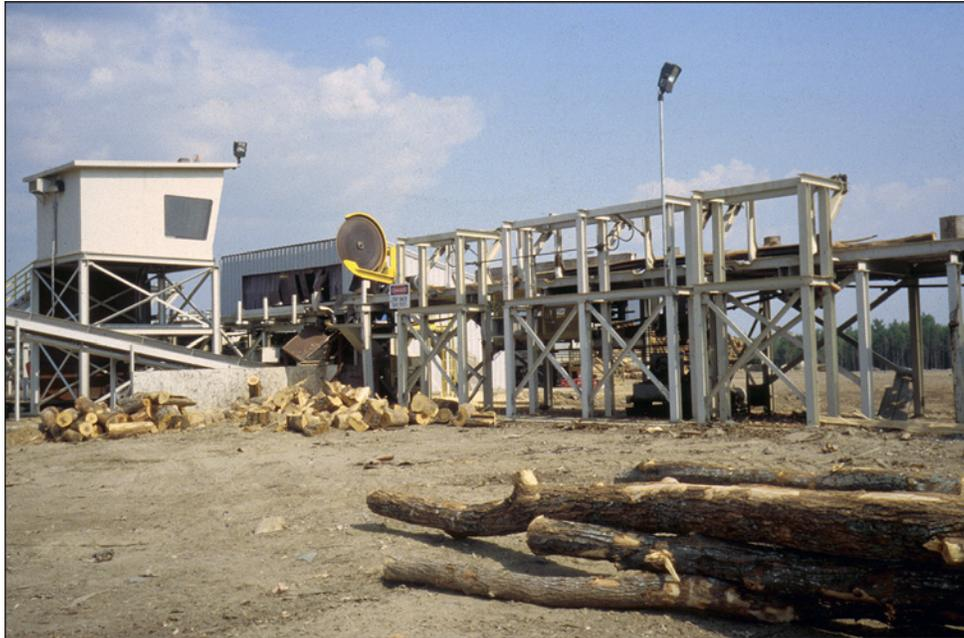
**Figure 6—Automated log merchandiser system for merchandising and sorting sawlogs from pulpwood material. (Photo by Rusty Dramm, USDA Forest Service)**
