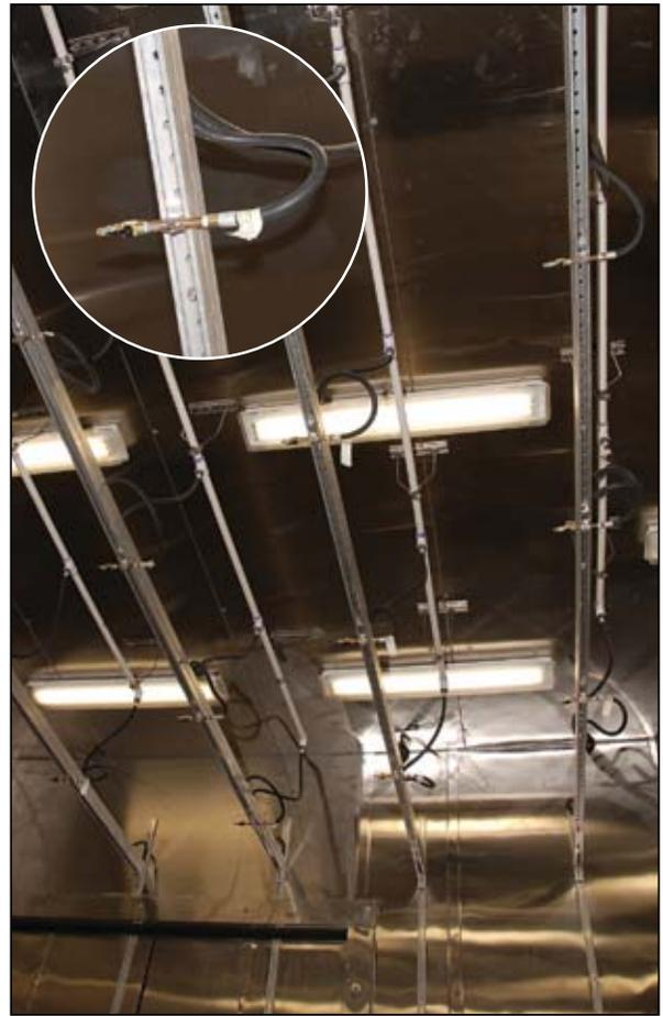
Partial view of rain nozzle array with inset close-up view. Water from rain simulation is collected, filtered, and reused in CARWASH tests.
