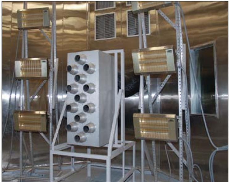
Infrared heat lamps and wind nozzle assembly inside the chamber.
