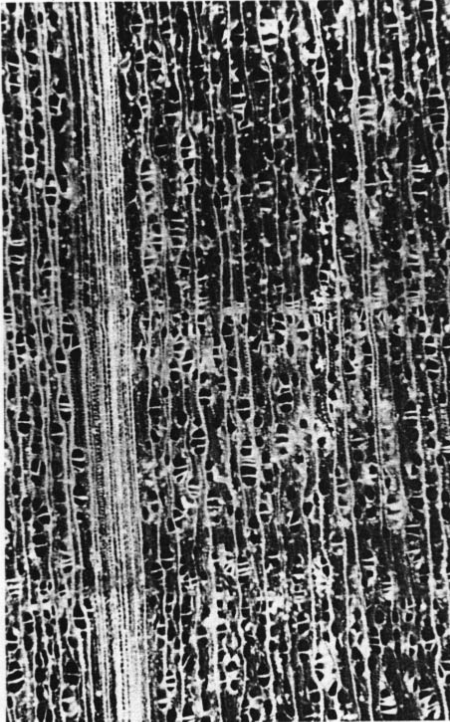
Figure 3—Wood of red alder magnified 15 times shows numerous small pores and simple rays, with an aggregate ray visible on the left. Photo by R. L. Krahmer, Oregon State University.
