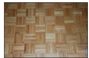
Several combinations of wood species were designed and laid out as test flooring on the FPL's fourth floor to measure effects of humidity, temperature change, and general use.
