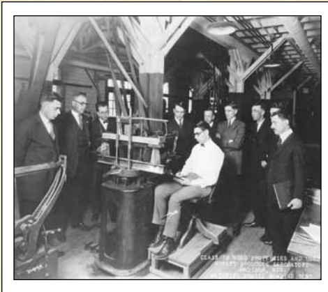
Students in an early Wood Properties and Uses course observe a static bending test to measure strength properties of wood.
