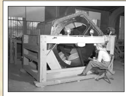
Testing box materials and construction for durability helped revolutionize the shipping industry during and after World War I.
