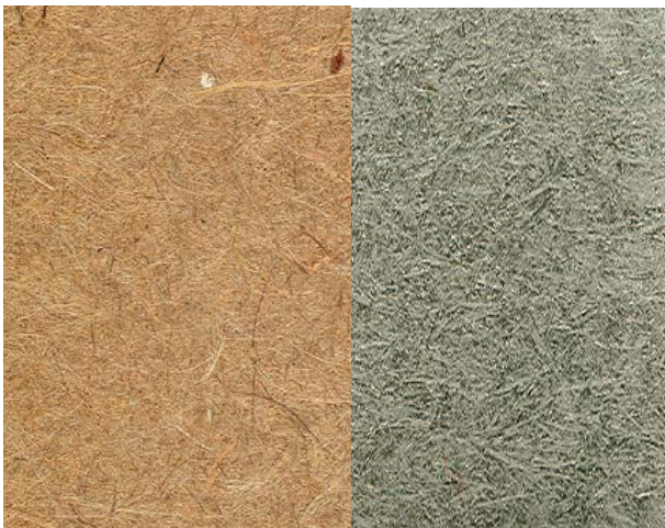
Figure 12 – Normal fiberboard surface (left) same fiberboard surface sputtered with aluminum (right).
