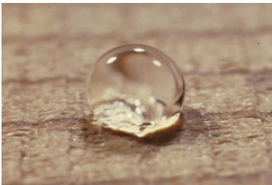
Figure 2 – Drop of water on a plasma treated surface.
