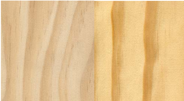
Figure 1 – Southern pine control (left) and plasma treated (right).
