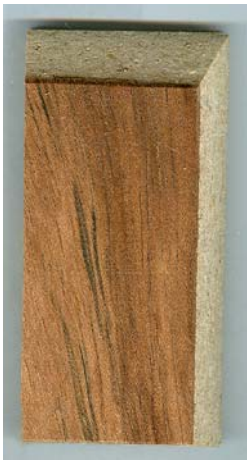
Figure 13 – Property enhanced surface veneer over low value core.
