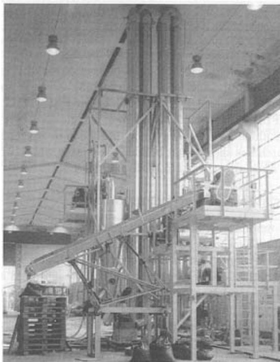
Figure 22.2. Fiber acetylation pilot plant in Sweden
