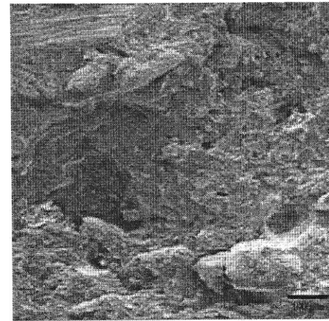
Figure 4. ~ SEM images of PLA-40% PWF: 100 \mu\text{m} (left, 0% silane) and 100 \mu\text{m} (right, 0.5% silane).
