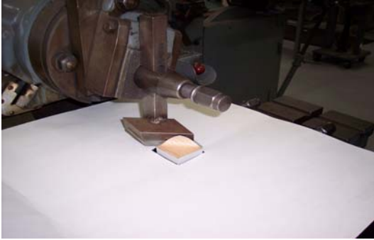
Figure 5. Slicing a thin wood layer with a microtome knife.
