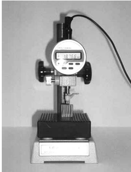
FIGURE 4.5 Measuring wood swelling using a flat-bed micrometer.
