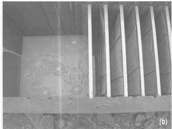
Figure 1. – Lignocellulosic filtration system: a) filtration box, b) filter frames inside filtration box.
