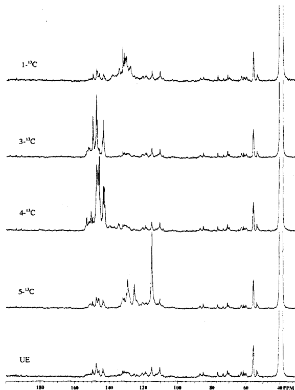
Fig 2. Quantitative ^{13}\text{C} NMR spectra of irradiated (2x21 h) 1-, 3-, 4-, and 5- ^{13}\text{C} DHP and unenriched (UE) DHP.
