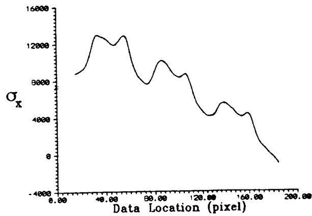
Figure 5—A smoothed, axial stress distribution plot over half the length of the plate.
