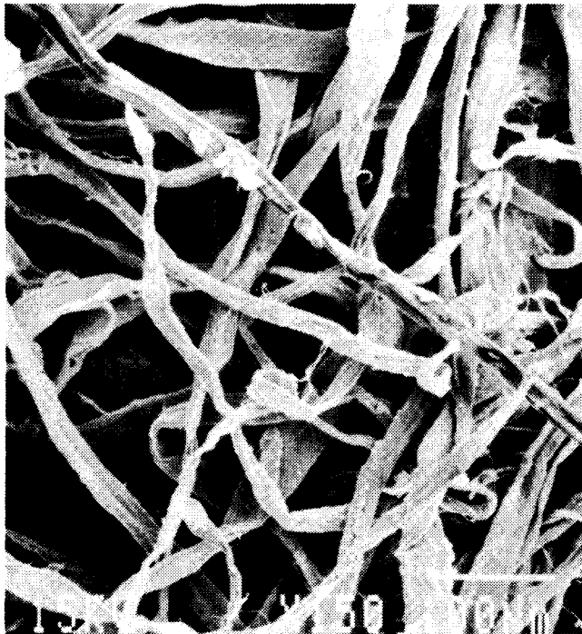
FIGURE 2: Recycled fibers after being dried and rewetted three times.
