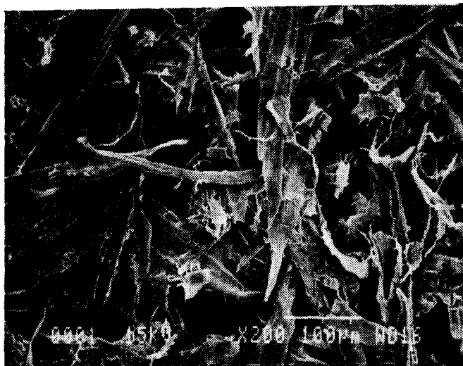
Figure 2—Electron micrograph of wet-formed handsheet made from unbeaten dry-fiberized newsprint.
