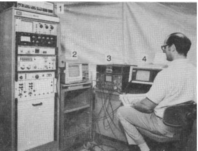
FIG. 4—Instruments for controlling force plate vibration, acquiring data, and determining transmissibility response of specimen. (1) Analog load cell summing amplifier. (2) Frequency analyzer. (3) Multichannel digital storage oscilloscope for recording time domain data. (4) High speed microcomputer with digital-analogue conversion ability for vibration control and analysis of storage oscilloscope data. (5) Signal conditioners.
