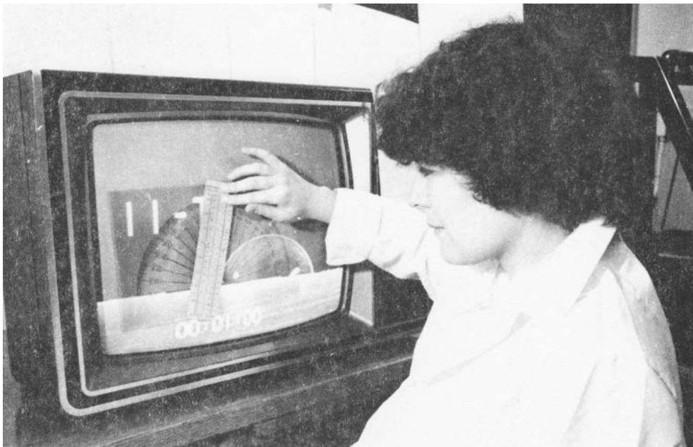
FIG. 2. Contact angle made by a drop of water on wood surface being measured from videotape image at 1-s elapsed time (M85 0405-12).
