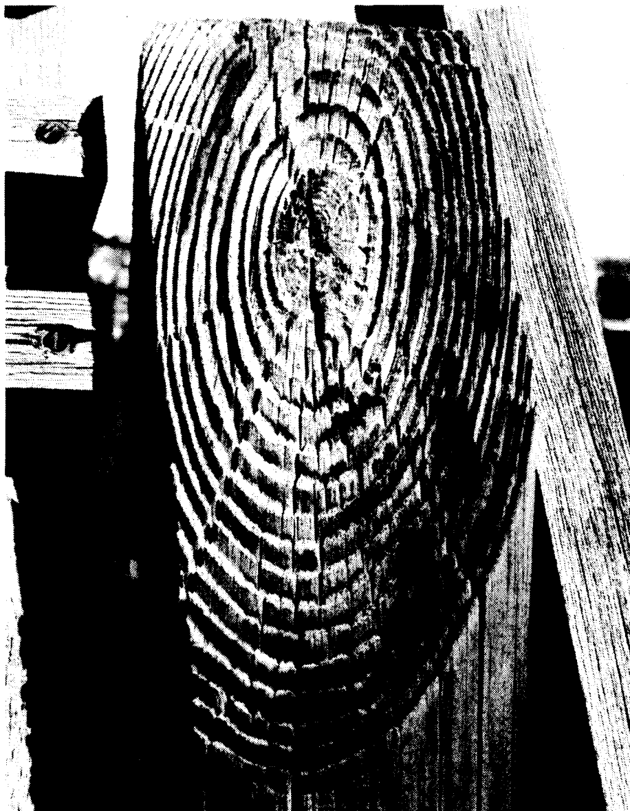
Figure 7. Weathered surface of softwood after 15 years of exposure in Madison, WI.
