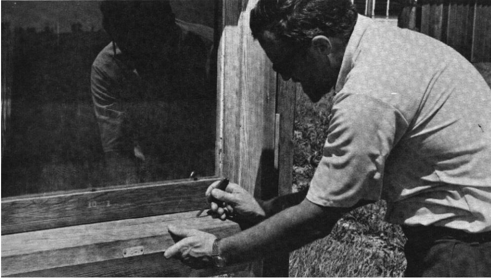
Figure 4. View of window unit protected for 20 years by dipping for 3 minutes in water repellent. Condition is as good as that with water repellent plus preservative.
