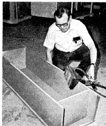
Fig. 1. Apparatus used to form handsheets varying in degree of fiber orientation. The mold was drawn through the slurry by hand.
