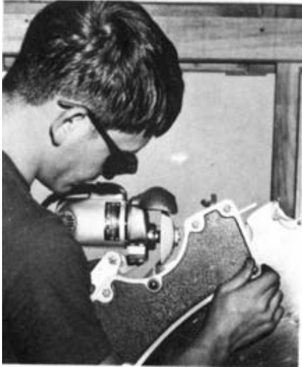
Figure 35. – An experienced operator can sharpen inserted sawteeth with an electric grinder in 3 to 5 minutes
