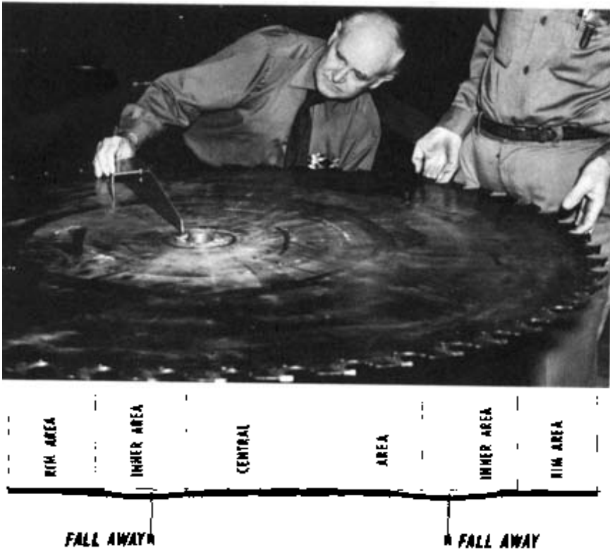
Figure 28. —A tension gage is used to measure amount of fall away (tension) in a circular saw.
