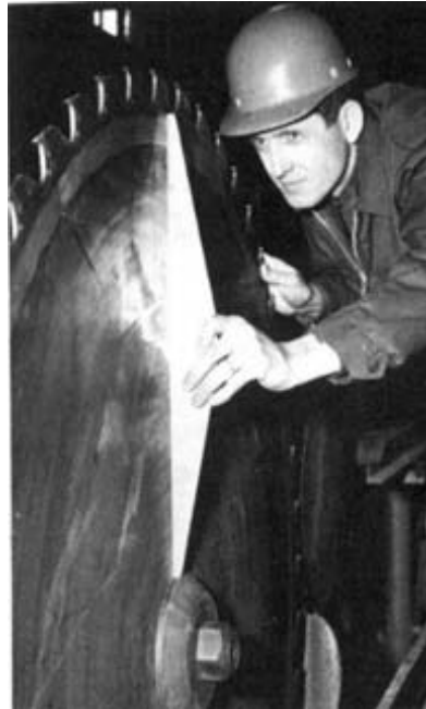
Figure 30.—Check log side of the saw for flatness with a machined straightedge.
