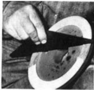
Figure 48. — Test for taper condition of saw collar by the following 3-step process: (A) first chalk the bearing surface. (B) scrape a machined straight-edge across the full face of the collar; if chalk is removed from the outer edge only, taper is all right. (C) if chalk is removed the full width of the bearing surface, taper is lacking.
