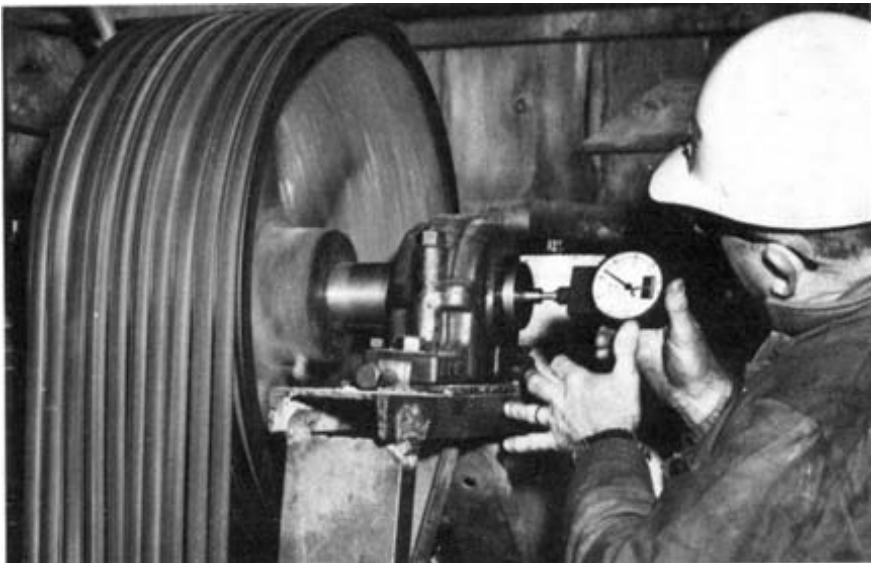
Figure 26. – A quick way to check saw speed is to use a direct-reading speed indicator.
