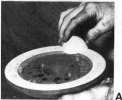
Figure 48. — Test for taper condition of saw collar by the following 3-step process: (A) first chalk the bearing surface. (B) scrape a machined straight-edge across the full face of the collar; if chalk is removed from the outer edge only, taper is all right. (C) if chalk is removed the full width of the bearing surface, taper is lacking.
