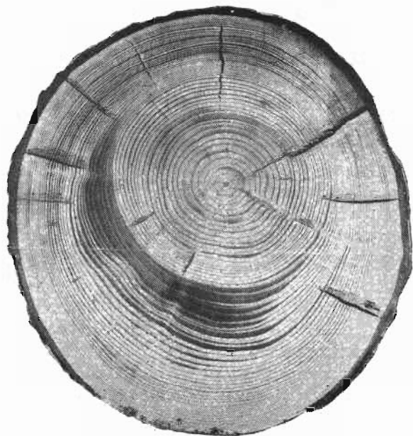
CROSS SECTION OF LOG CONTAINING COMPRESSION WOOD
