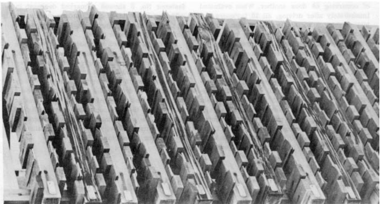
Figure 9.--Test specimens after 1-year's exposure at the U.S. Forest Products Lab. exposure site west of Madison, Wis. Note the weathered appearance and the deterioration of the plywood cover pieces.
