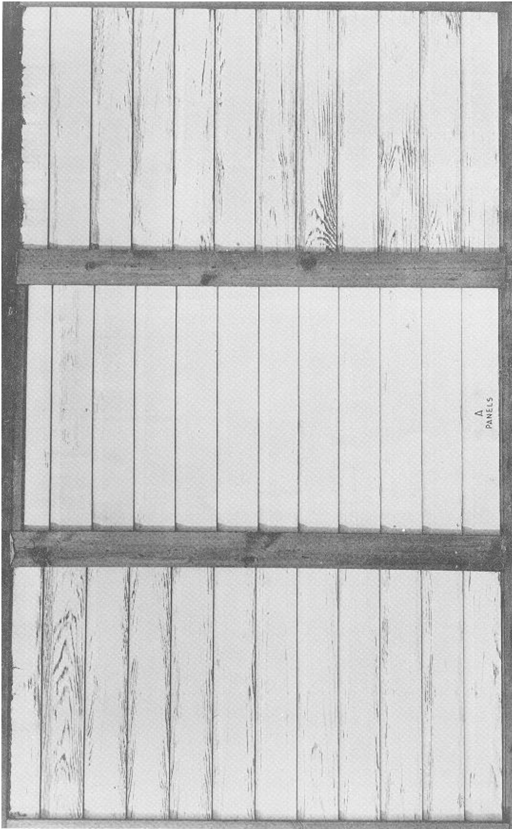
Figure 6. --Exterior view of panels A (southern yellow pine) (left A-1, center A-2, and right A-3) Center panel was treated and end panels were untreated. The difference in paint retention can be noted. All siding was flat-grained. Panels had been exposed for 3 years
