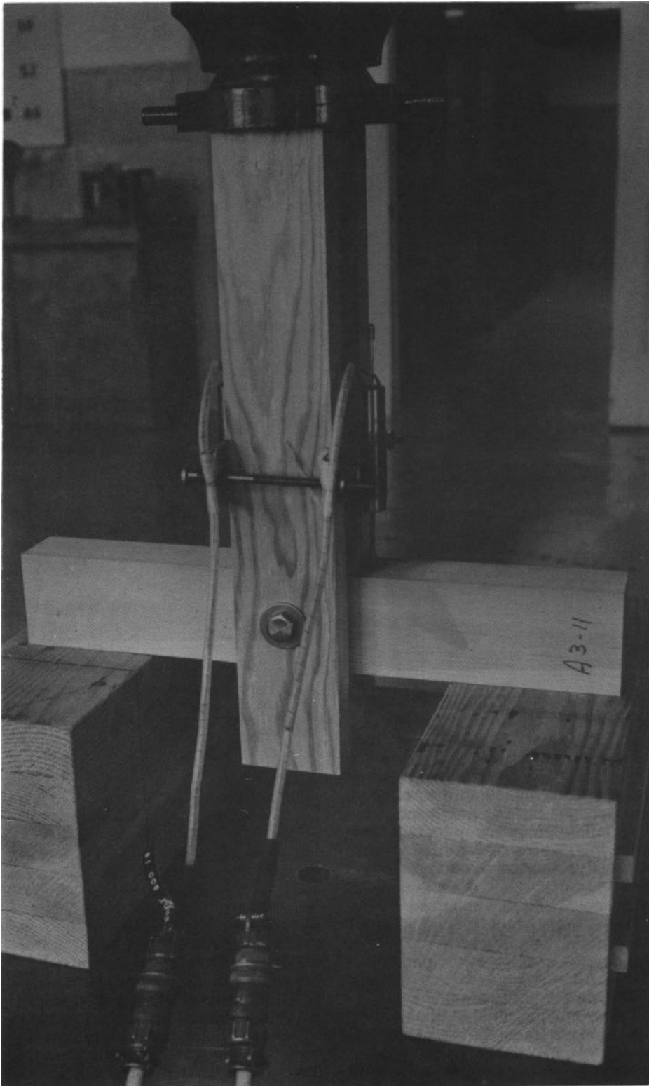
Figure 8.—Loading bolts perpendicular to the wood grain with average load as Percent Of solid wood load and theoretical load as percent of experimental load.
