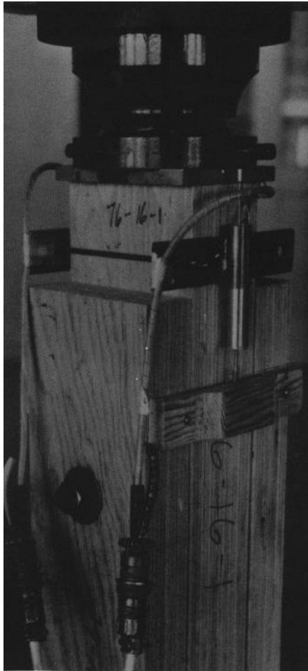
Figure 9.—Loading split-ring connectors parallel to the wood grain.
