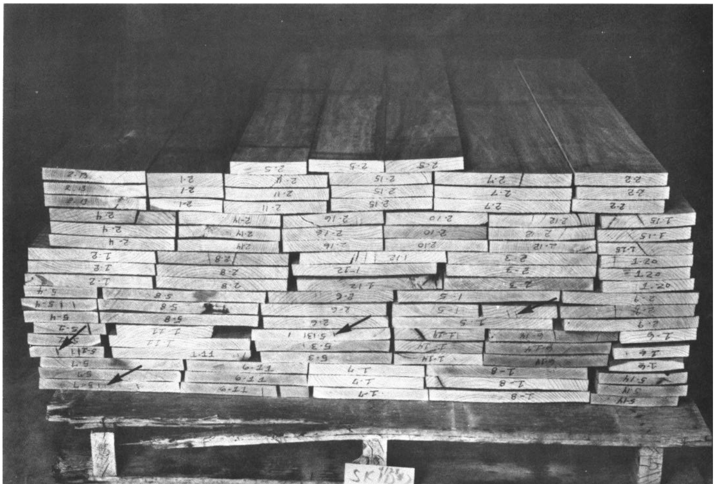
Figure 7.—Ends of oak lumber show honeycomb (arrows indicate typical examples) after accelerated kiln drying.
