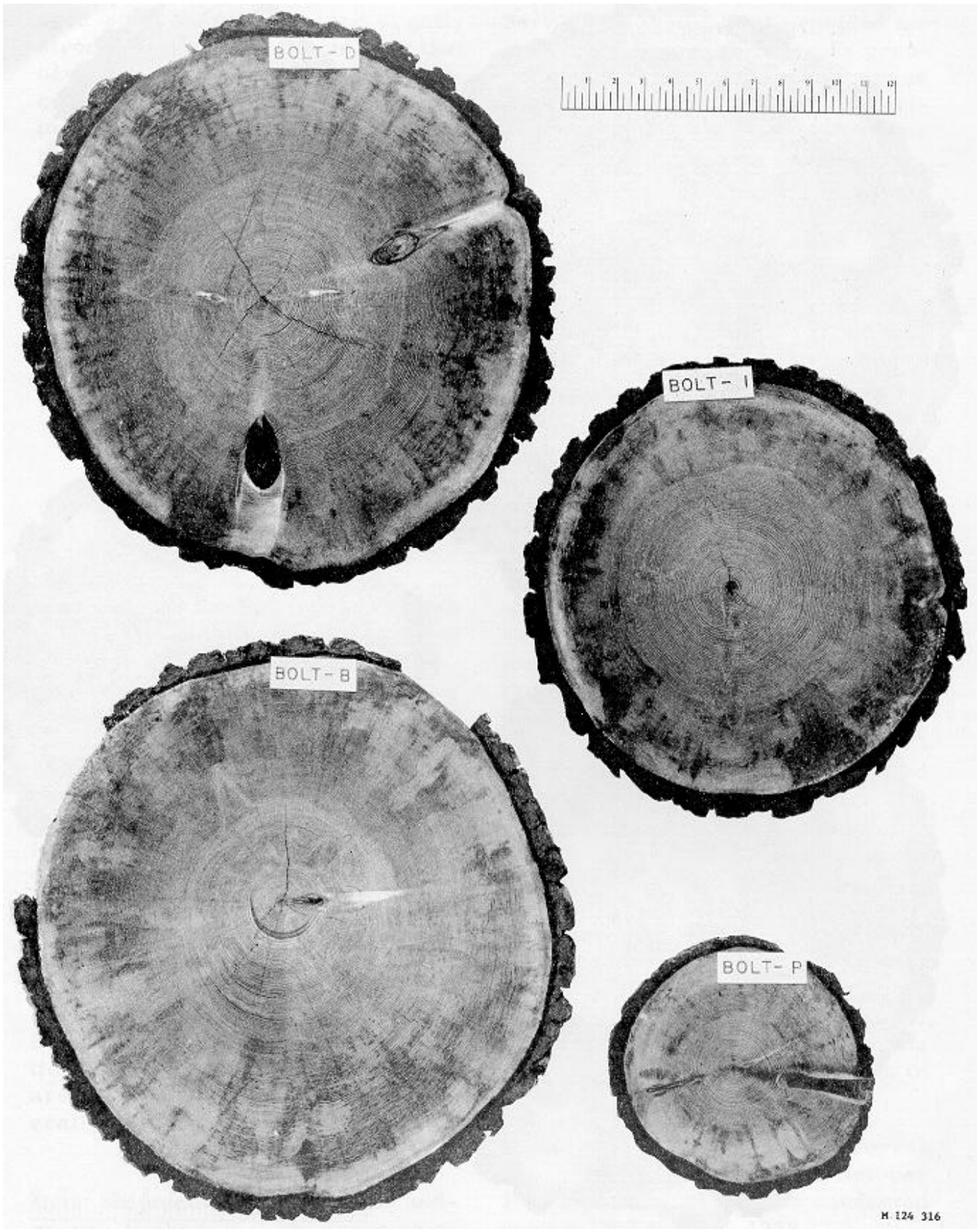
Figure 2. --Cross sections of a tree from Douglas County, Oreg., at heights of 4, 12, 32, and 60 feet. Only limited areas of compression wood are noticeable (bolts b and d ) and there is generally uniform growth throughout the height of the tree (bolts i and p ).
