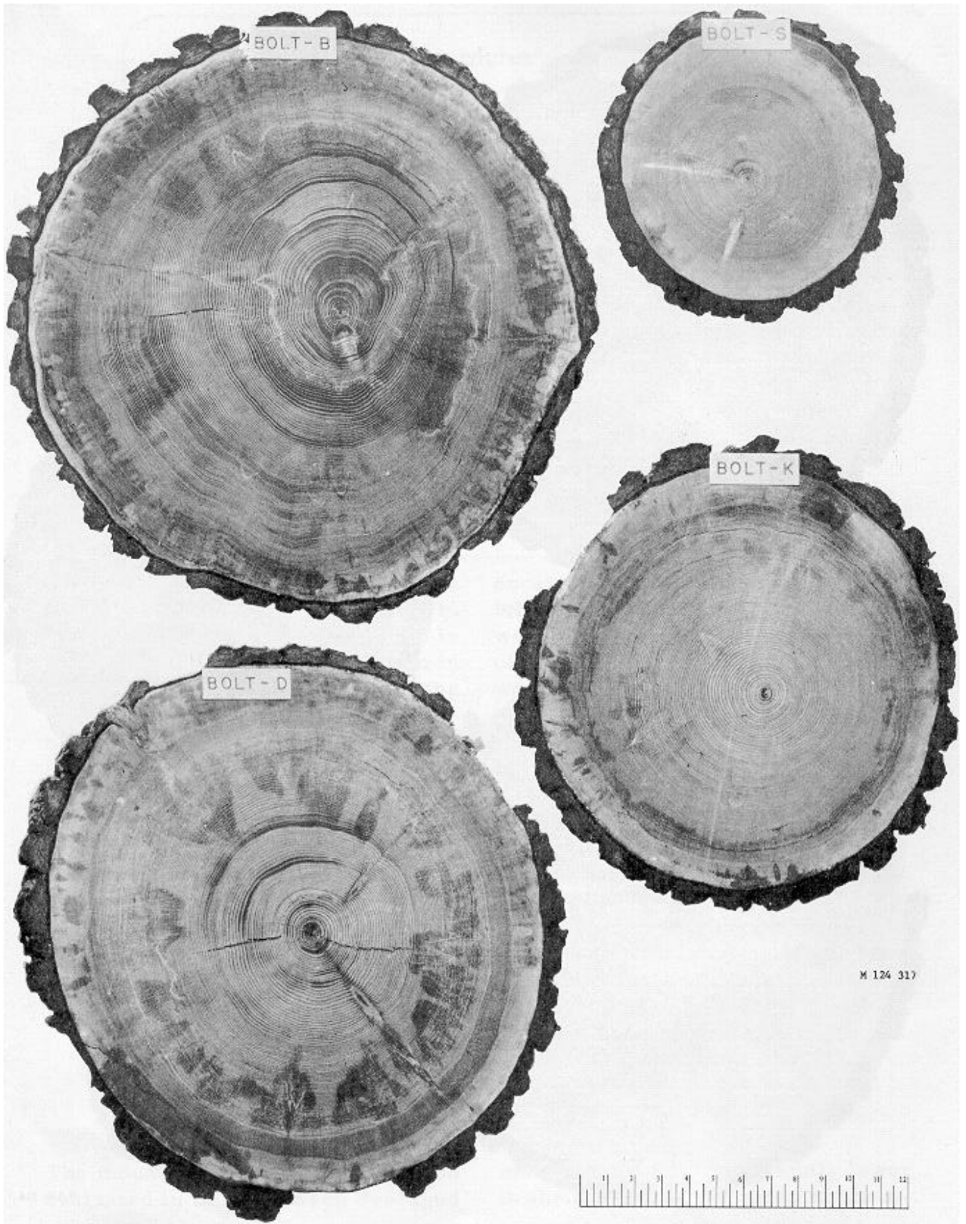
Figure 1.--Cross sections of a tree from Hood River County, Oreg., at heights of 4, 12, 40, and 72 feet. Compression wood (characterized by wide, dark, summerwood bands) is apparent in b and d , and uniform, clear growth can be observed in the wood higher in the tree (bolts k and s ).
