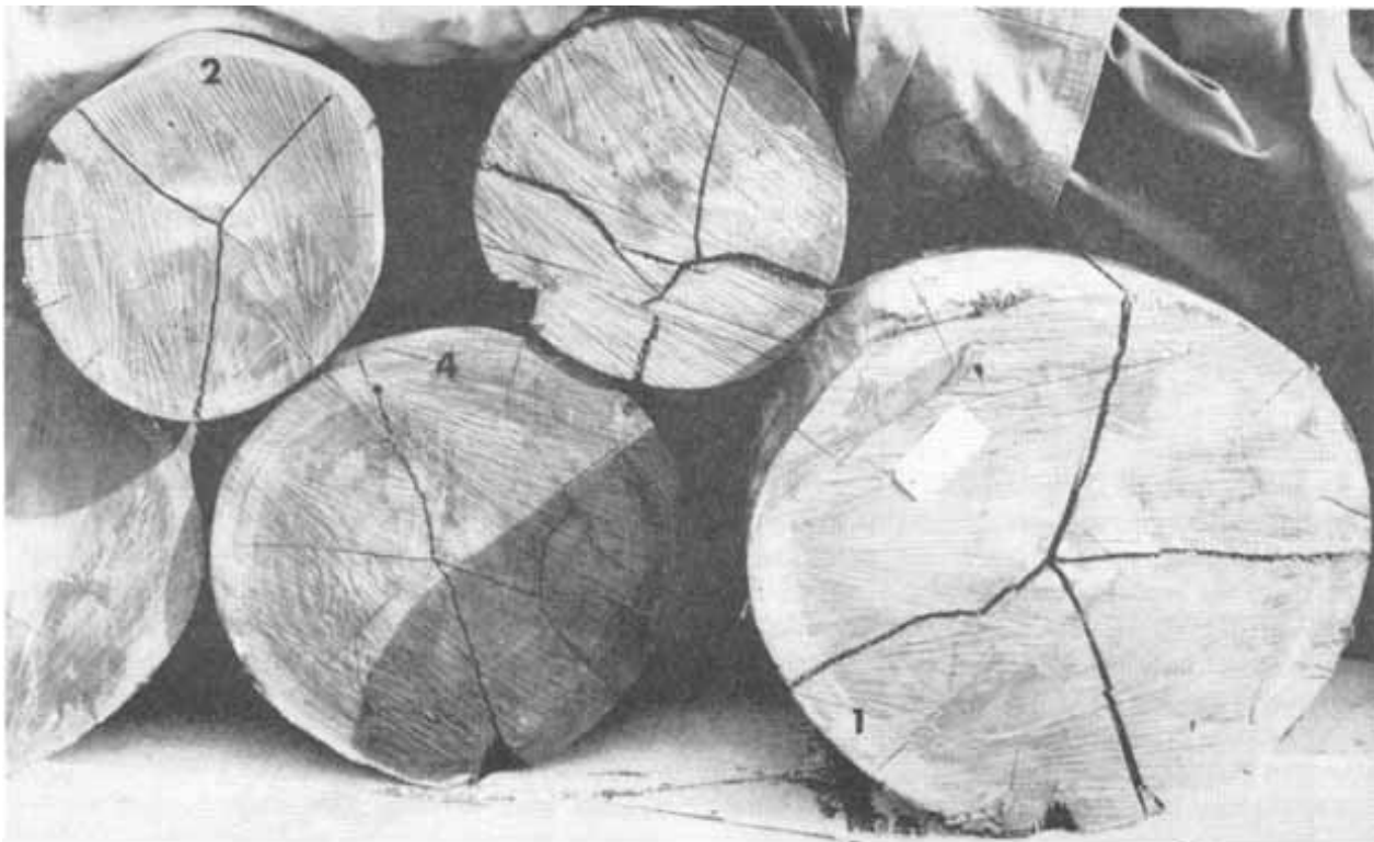
Figure 2.--End splits and checks in saligna eucalyptus bolts from Wood Valley site about 1-1/2 months after felling. Identified bolt-ends correspond to those shown on the left in figure 1.
