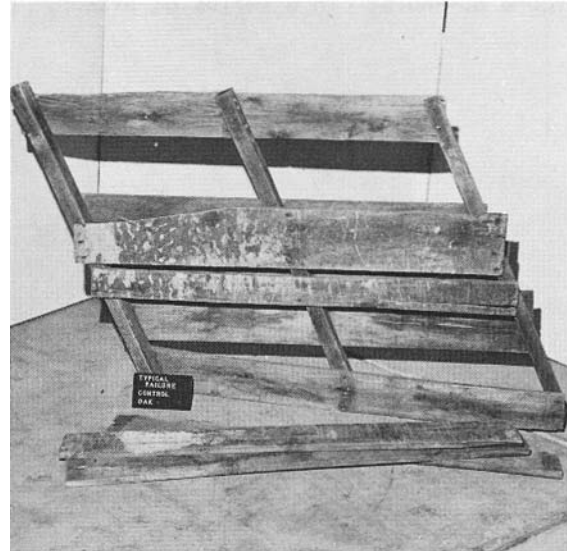
Figure 11.--An oak, three-stringer (control) pallet showing racked condition at failure. (M 138 570-4)
