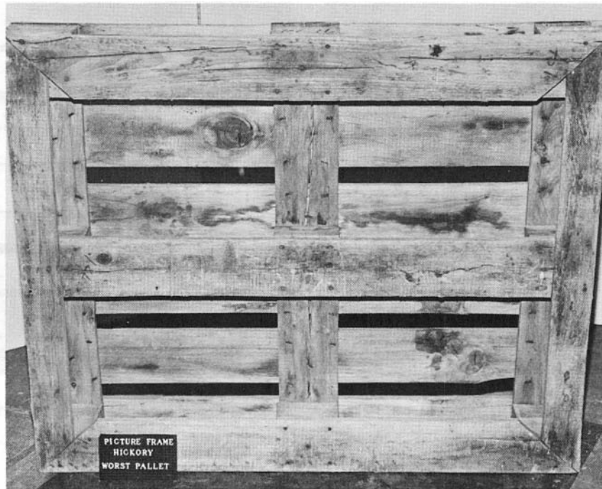
Figure 6.--Worst in a series of hickory, picture-frame pallets after 4 years of service. (M 138 347-5)
