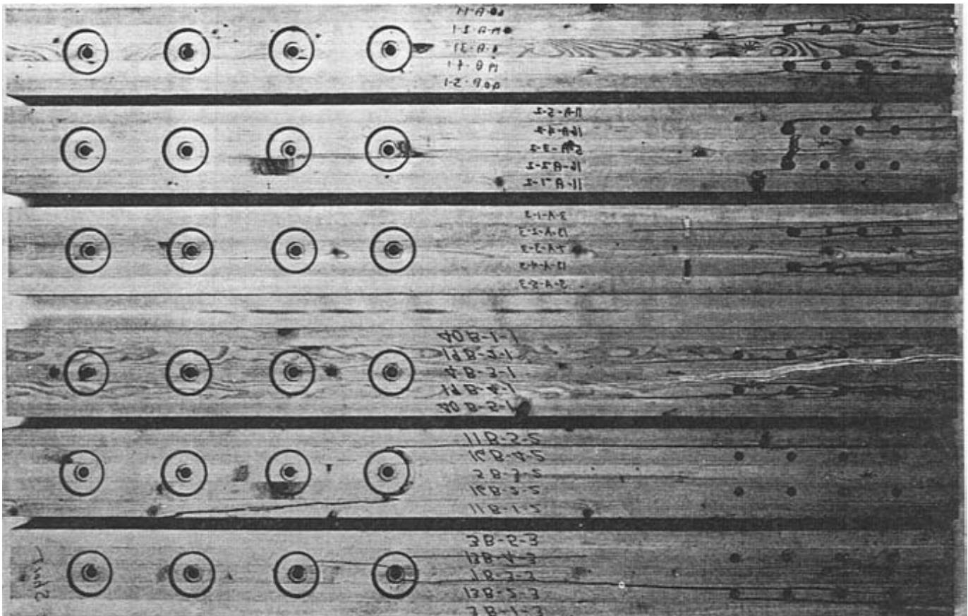
Figure 10.--Joints with eight 3/4-inch bolts after test. The upper three are series A specimens with 3-inch spacing between bolts and the lower three are series B specimens with 4-1/2-inch spacing between bolts. End distance in all tests was 5-1/4 inches.
